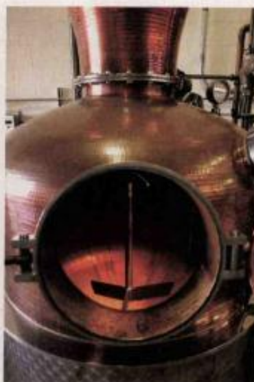
ABOVE, FROM LEFT: The father-and-son team of Bob and Doug Ryan produce small-batch vodka, rum, gin, and rye whiskey at Ryan & Wood Distilleries in Gloucester, Massachusetts; their 600-liter copper alembic pot still was custom-made in Germany; small casks hold experimental batches.
